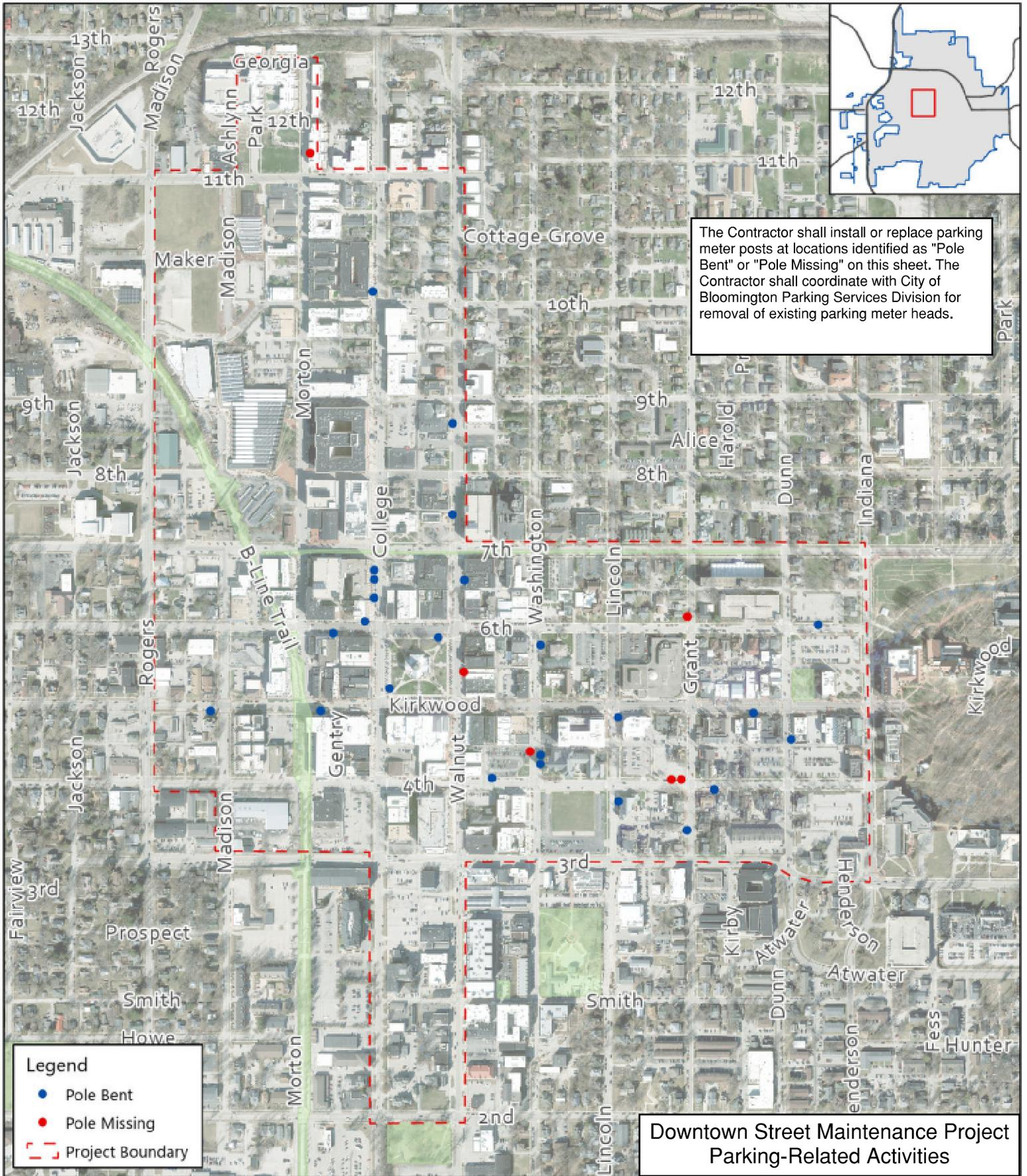
The Contractor shall install or replace parking meter posts at locations identified as "Pole Bent" or "Pole Missing" on this sheet. The Contractor shall coordinate with City of Bloomington Parking Services Division for removal of existing parking meter heads.
