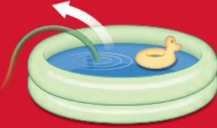
Any hose is a cross-connection when left submerged in a swimming pool, laundry sink, or car wash bucket.
